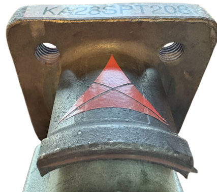
Figure 2. TDG-Coated Station Post End Fitting after ANSI/NEMA C29.11 Tracking Wheel Testing and CSA C156.2 Steep-Front Impulse and Power Frequency Voltage Testing
