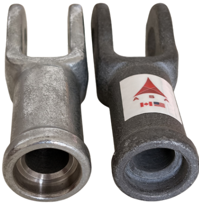
Figure 1. Comparison of Internal Corrosion Protection in Deadend/Suspension Insulator Clevis Fittings: Conventional HDG vs ArmorGalv® TDG
